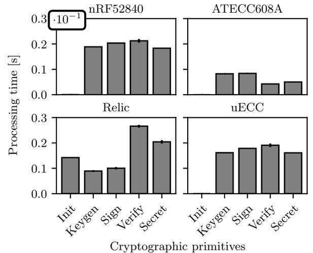
**Figure 4. Processing time of different elliptic curve algorithms. Crypto-operations are either accelerated in hardware on the microcontroller (nRF52840), on an external chip (ATECC608A), or in software (Relic, uECC).**
