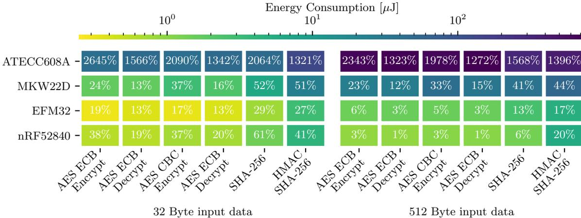
**Figure 3. Energy consumption of hardware accelerated cryptographic operations on different platforms. Percentages show relative overhead compared to crypto-implementations in software running on the same devices.**
