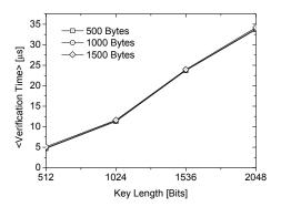
Fig. 1. Processing times for CGI signature verification
