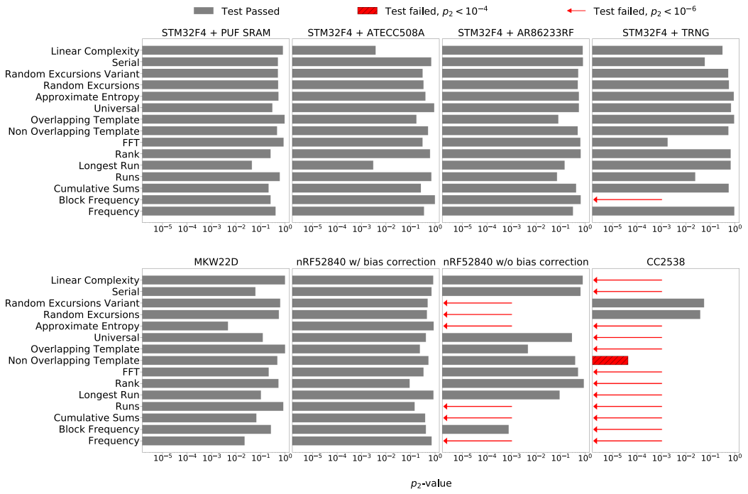
Fig. 1. Hardware-generated random numbers: \chi^2 -test results on the distribution of probability values from 15 NIST STS tests. p_2 -values \geq 0.0001 pass the hypothesis of uniformity.
