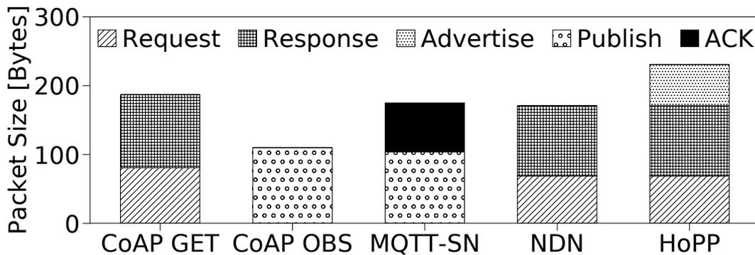
Figure 3.2: Packet sizes in bytes for each protocol.
