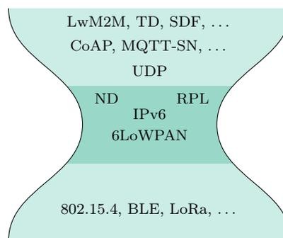
Figure 1.1: Building blocks and protocols to form an IoT network stack.
