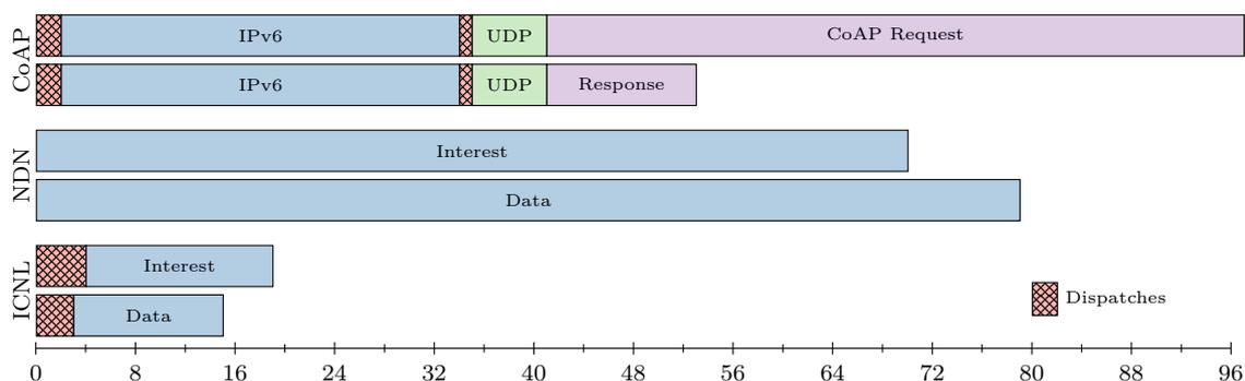
Figure 4.7: Packet length and structure for different protocols.
