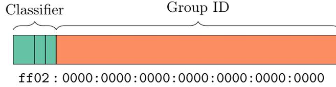
Figure 9.6: IPv6 link-local multicast address format [258] using a 2-byte classifier and a 14-byte group id.
