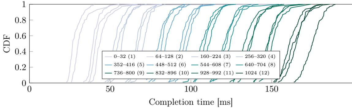
Figure 4.14: Temporal distributions of content arrival times for different payload sizes in bytes. The amount of fragments is given in parentheses.
