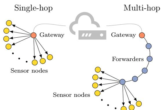
Figure 9.8: Topologies for single-hop and multi-hop experiments.
