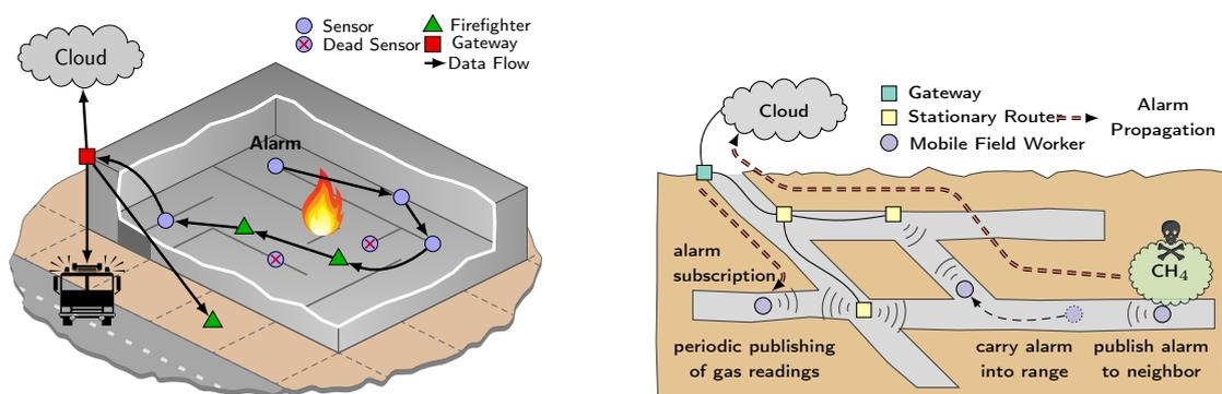
(a) Resilient machine-to-machine communication for the Industrial IoT with heterogeneous constrained IoT devices. (b) IoT use cases in industrial settings with device mobility and network partitionings.
