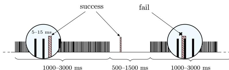
Figure 4.16: Radio interference due to bursty cross-traffic.
