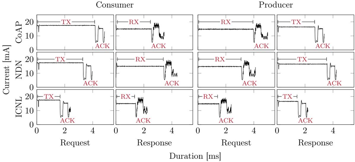
Figure 4.11: Current consumption for send and receive operations.
