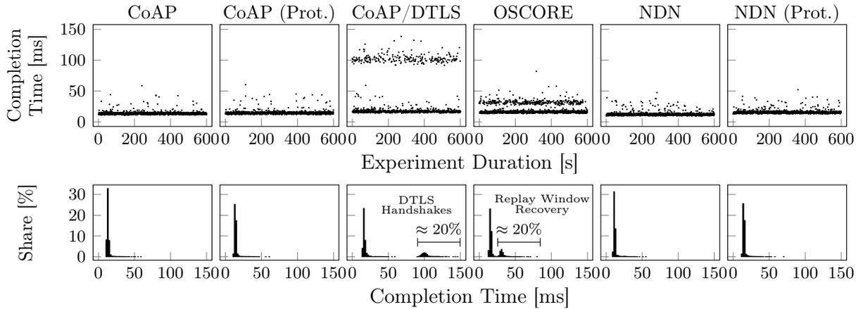
Figure 9.10: Content arrival times and their percental distribution during the evolution of an experiment in a single-hop scenario, with simulated reboots after 20% of all exchanges. DTLS and OSCORE clearly reflect these events as delayed handshakes or replay window recovery, respectively.
