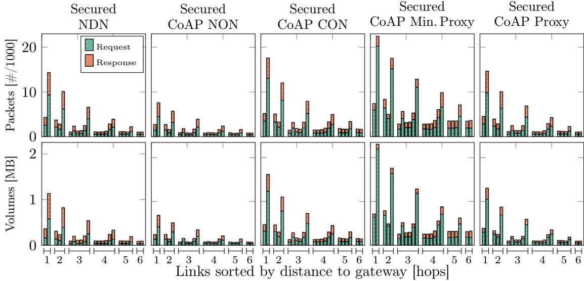
Figure 10.5: Number of packets and bytes transmitted over the air per downstream and upstream link in the topology for each deployment with security measures enabled.
