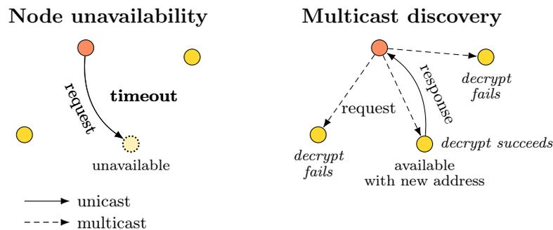
Figure 9.5: Node discovery with OSCORE using a scoped multicast request.
