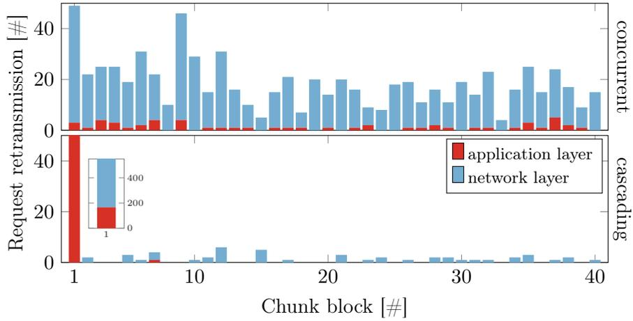
Figure 8.14: Chunk request retransmissions on the application and network layer grouped into blocks of 100 chunks for the  $n_7$  node.
